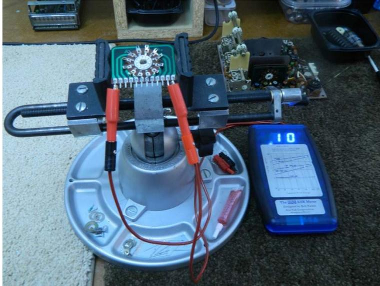
Each contact is checked for high resistance after cleaning. I am using here the Blue ESR meter which will measure quite low resistances. The reading here is .1 ohm. As you get closer to the other probe, the resistances will decrease as it is reading the resistance of the traces on the board. I also check physically for any looseness of the contact on the board. These contacts are originally held in place with rivets and they sometimes loosen.
