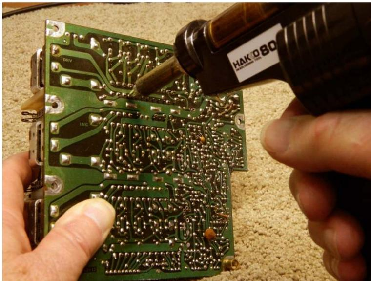
Using the Hakko 808, it is a simple matter to remove the solder around each wafer pin completely. When you have removed the solder from each pin, the wafer will fall out of the board.
