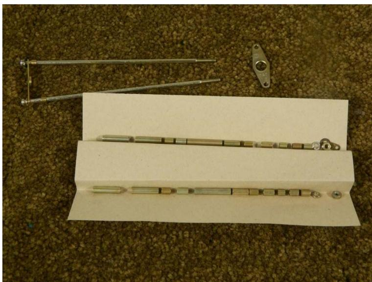
These are the through screws and spacers as removed from the switch assembly.
